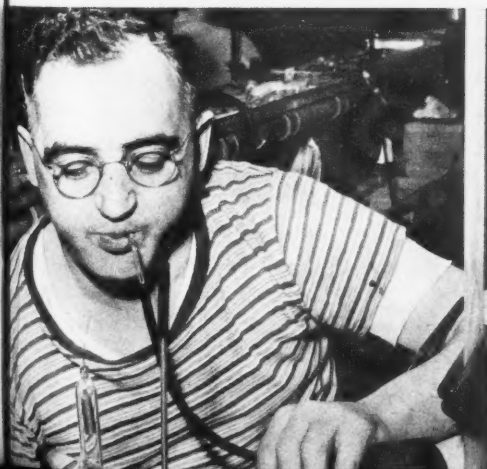
To splice two ends of glass tubing together into a perfect circle, the blower uses a special torch. Below, craftsman puts the electrode in the tube.
